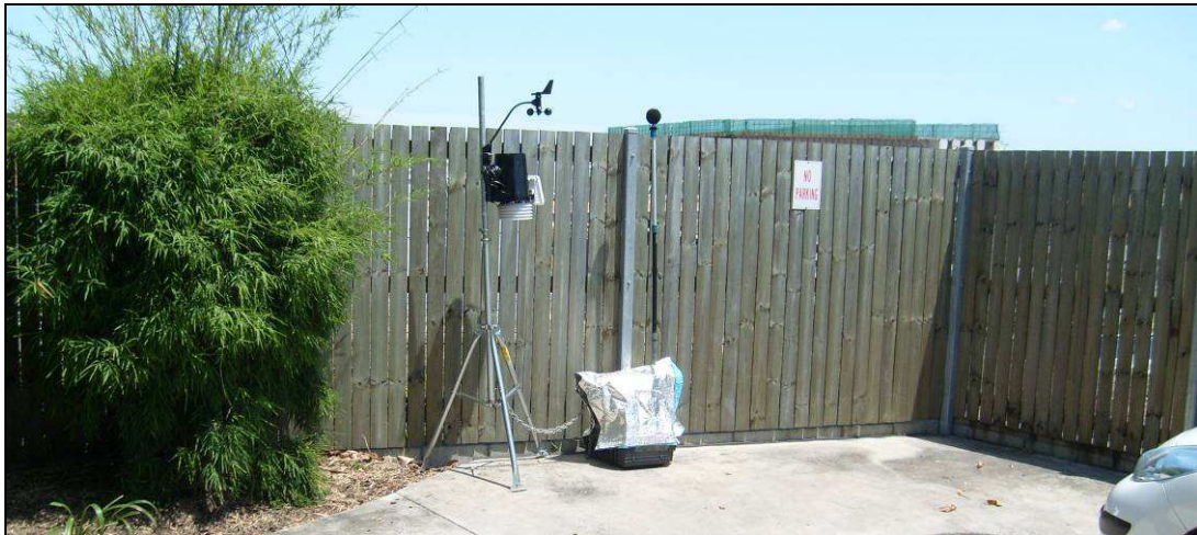
Photo A3: ML3 – Noise logger at 6 Tufton Street, Bowen Hills.
